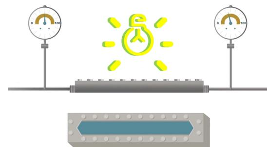
Fig. 9: HANU reactor built for the thiol-ene click reaction.
