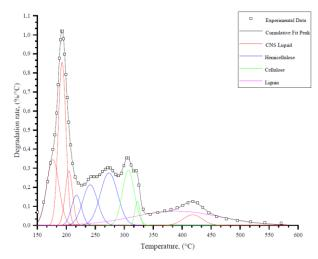
**Figure 2.** Gaussian deconvolution of DTG curve from thermogravimetric analyses performed under high-resolution approach (initial heating rate: 30 °C/min; resolution: 5; sensitivity: 1.0) for raw cashew nut shell. The graph shows the deconvoluted peaks for hemicellulose (blue), cellulose (green), lignin (pink) and cashew nut shell liquid (red). Temperature range selected from 150 to 600 °C. Coefficient of determination (r<sup>2</sup>): 0.9994.
