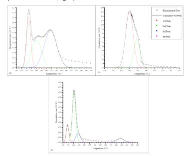
**Figure 1.** Gaussian deconvolution of DTG curves from thermogravimetric analyses performed under high resolution approach (initial heating rate of 30 °C/min; sensitivity 1.0; and resolution 5.0) for (a) xylan, (b) microcrystalline cellulose (MCC) and (c) cashew nut shell liquid (CNSL). Coefficient of determination ( $r^2$ ): a) 0.961, b) 0.994 and c) 0.997.
