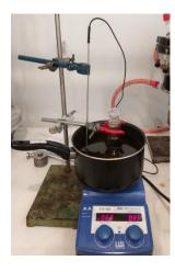
Figure 2. Batch reactor used in the experiments.
