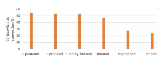
Figure 3. Extent of esterification of the bio-oil at 40 °C using different types of alcohol and 5% of catalyst.
