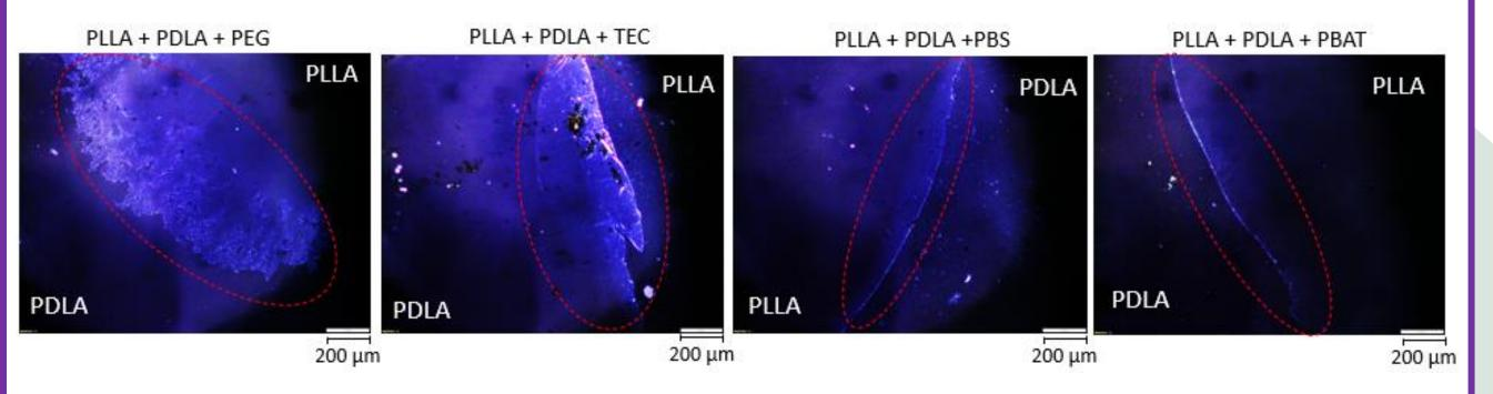
Figure 2. Effect of each plasticizer/polymer on the stereocomplexation of PLLA and PDLA after 10 min of contact in the polarized light microscope with hot stage
