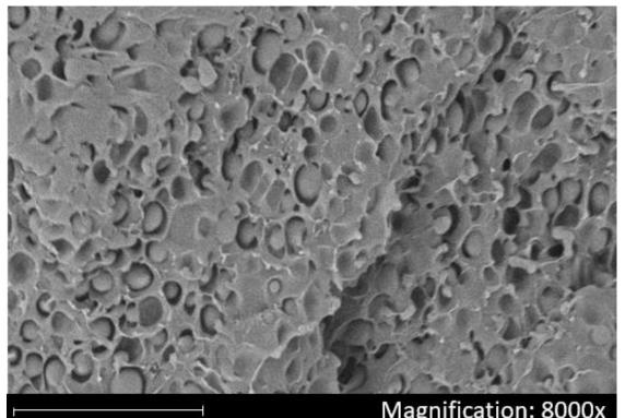
Figure 3 shows the presence of two different phases when blending PDLA and PBAT. This same behavior is observed for all samples with PBAT or PBS.
