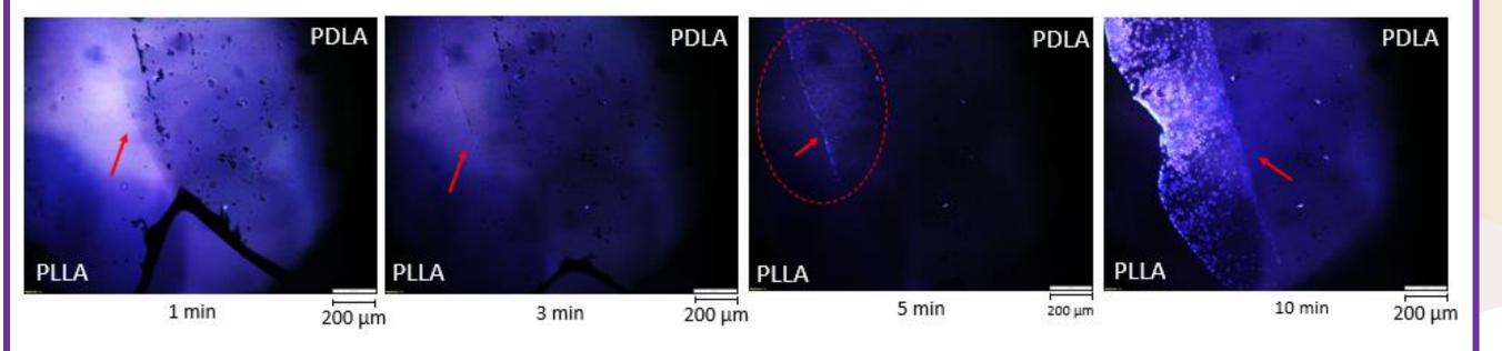
Figure 1. PLLA-PDLA behavior under polarized light microscope upon heating the sample at 200 °C for 10 minutes
