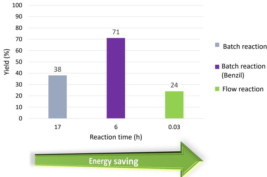
significantly higher yield was found (fig 8). Lastly, the reaction was performed in continuous flow using the Labtrix Start reactor Despite the set up. relatively lower yield, the result is promising, achieved within a short reaction time of 0.03 h.
